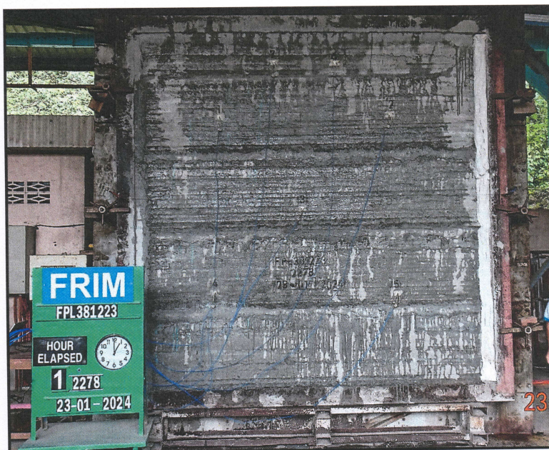
Plate 5. During fire resistance test (Time taken: 60 minutes).
