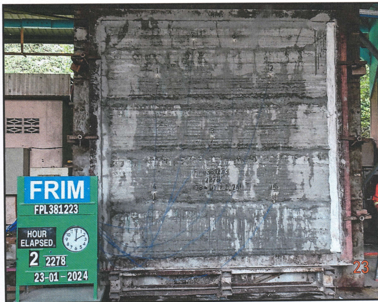
Plate 7. During the fire resistance test (Time taken: 120 minutes).
