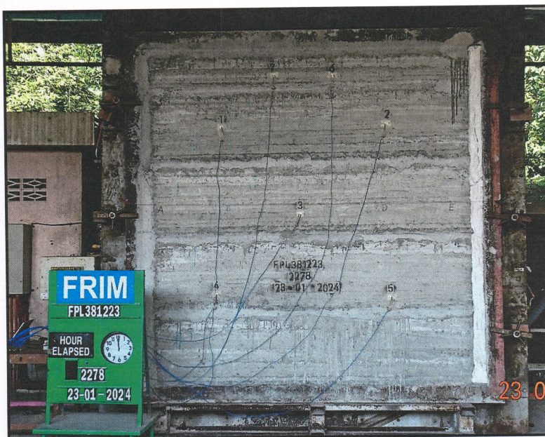
Plate 3. Before the fire resistance test (Time taken: 0 minutes).
