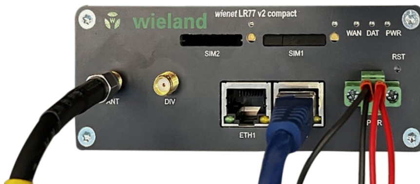
*Illustration 3: Visualization of the batch plant's router.
