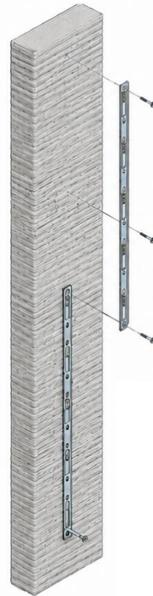
Figure 2 Installation of wall ties
